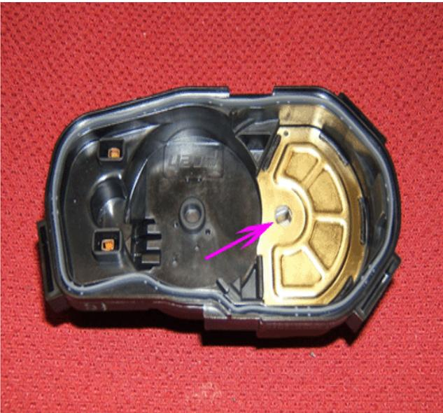
16. Place the TP sensor cover in the position as shown. Confirm the TP sensor drive slot orientation is aligned in the TP sensor cover as shown.
