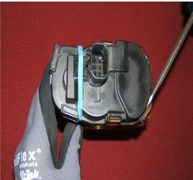
Notice DO NOT PRY ON THE MACHINED SEALING SURFACE OF THE THROTTLE BODY INLET DUCT.
