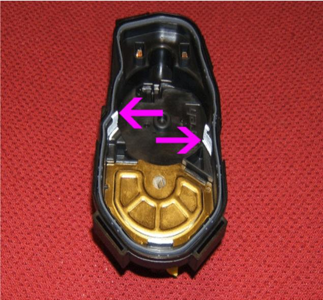
Notice The three TP sensor cover alignment tabs are highlighted in white for identification purposes only.
