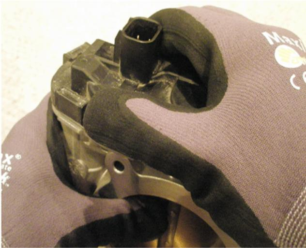
11. Hold the throttle body with your hand, so that the TP sensor cover is facing upward. Grasp the TP sensor cover and carefully lift it up and separate it from the throttle body.
