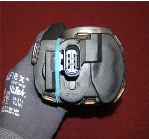
8. Secure a rubber band around the throttle body and TP sensor cover as shown.
