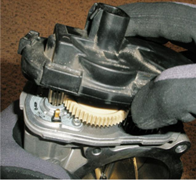
21. Position and install the TP sensor cover to the throttle body. Hold the TP sensor cover in position. If necessary for ease of the clip installation, secure a rubber band around the throttle body and TP sensor cover.
