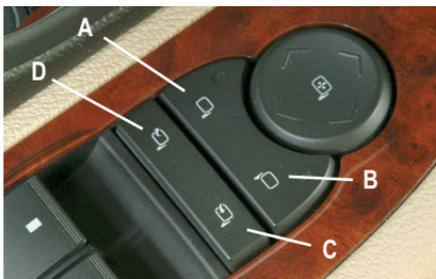
The following power foldaway mirror controls are located on the driver's door:
