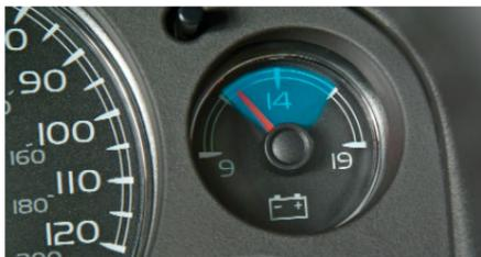
The voltmeter shows the condition of the vehicle's charging system. The system is designed to regulate voltage output to help improve fuel economy and extend battery life. Normal system operation readings may fluctuate (as indicated by the blue area in the illustration above) based on vehicle operation, including the number of electrical accessories being operated and engine speed.
