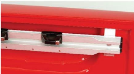
The rails are notched at each end to allow the tie-downs to be removed and placed on another rail. To remove, pull out the locator pin and slide the tie-down to the end of the rail and pull back.
