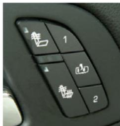
**(Heated Seatback):** Press the top button to turn on the heated seatback.
