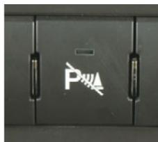
To turn off the system, press the
