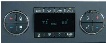
The automatic climate control system maintains the desired individual temperature for the driver and front seat passenger. The system adjusts the airflow mode, fan speed, air conditioning and recirculation functions to reach the set temperature(s) as quickly as possible.
