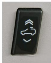
**Vent:** From the closed position, press and hold the rear of the switch to vent the sunroof.
