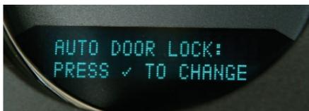
Your vehicle's Driver Information Center (DIC) provides vehicle information, vehicle feature customization (if equipped), and vehicle warning messages. The DIC messages will be shown on the instrument panel cluster display.
