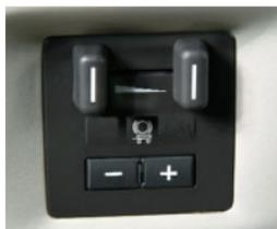
electric trailer brakes and to manually apply the trailer brakes. ITBC system information is displayed on the Driver Information Center.
