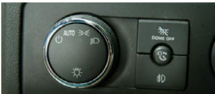
The exterior and interior lamp controls are located on the instrument panel to the left of the steering wheel.
