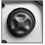
If your vehicle has this feature, the four-way control is located on the outboard side of the seat.
