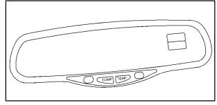
The mirror also includes a display in the upper right corner of the mirror face. The compass reading and the outside temperature will both appear in the display at the same time. The dual display can be turned on or off by briefly pressing either the TEMP or the COMP button.
