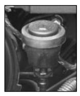
The clutch master cylinder reservoir is located in the rear of the engine compartment on the driver's side of the vehicle. See "Engine Compartment Overview" in the Index for more information on location.
