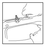
Insert a tool into the push-pin slot and pull downward until the push-pin snaps loose.
