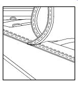
1. To remove, unsnap the cover. Roll up and stow using the buckle and the strap located at the front of the box.
