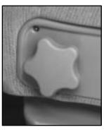
If your vehicle has a lumbar adjustment, the knob is located on the outboard side of the seat cushion.
