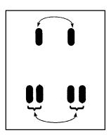
If your vehicle has dual rear wheels and the tread design for the front tires is different from the dual rear tires, always use the correct rotation pattern shown here when rotating your tires. The dual tires are rotated as a pair, and the inside rear tires become the outside rear tires.
