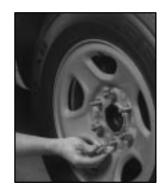
6. After mounting the spare, reinstall the wheel nuts with the rounded end of the nuts toward the wheel. Tighten each wheel nut by hand using the wheel wrench until the wheel is held against the hub.
