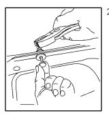
While continuing to pull downward on the push-pin, squeeze and turn the expandable end of the push-pin with a tool until it releases from the retainer.
