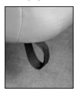
Pull forward on the release strap located under the rear seat cushion.
