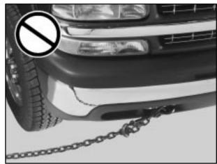
Your vehicle may be equipped with recovery hooks. The hooks are provided at the front of your vehicle. You may need to use them if you're stuck off-road and need to be pulled to some place where you can continue driving.
