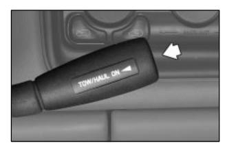
Your vehicle is equipped with a tow/haul mode. The selector button is located on the end of the column shift lever. You can use this feature to assist when towing or hauling a heavy load. See "Tow/Haul Mode" in the Index for more information.
