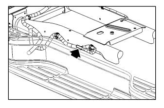
The six-wire harness is located at the rear of the vehicle and is tied to the vehicle's frame. The harness requires the installation of a trailer-wiring harness connector, which is available through your dealer.
