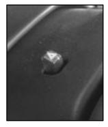
The hazard warning flasher button is located at the top of the steering column.
