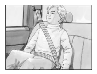
Buckle, position and release the safety belt as described in "Rear Seat Passenger Positions (Extended Cab and Crew Cab)" earlier in this section. Make sure that the shoulder belt crosses the shoulder.
