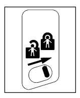
Your vehicle may have one of the two child security lock labels shown. This feature is located on the inside edge of the rear doors.
