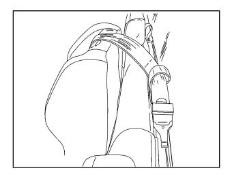
When using a child restraint with a top strap in the center rear position, route the top strap through the fabric loop on the seatback. Then, raise the head restraint and attach the top strap to the anchor point located at the closest outboard position.
