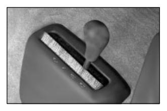
The transfer case shift lever is on the floor to the right of the driver. Use this lever to shift into and out of four-wheel drive. 4WD
