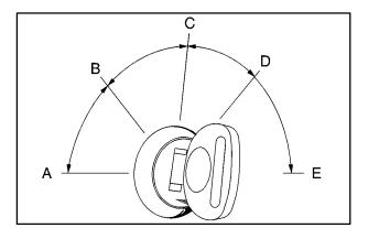
A (ACCESSORY): This position allows you to use things like the radio, power windows and the windshield wipers when the engine is off. Push in the key and turn it toward you.
