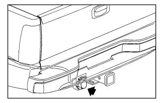
Your pickup may be equipped with the eight-wire trailer towing harness. This harness with a seven-pin universal heavy-duty trailer connector is attached to a bracket on the platform hitch.\*
