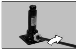
Turn the wheel wrench clockwise to raise the jack lift head a little.
