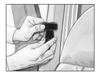
1. Remove the guide from its storage clip on the interior body.
