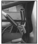
9. Now connect the black negative (-) cable to the negative (-) terminal of the good battery. Use a remote negative (-) terminal if the vehicle has one.
