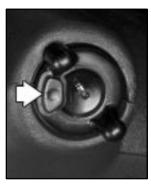
The ignition key cannot be removed from the ignition of manual transmission vehicles unless the key release button is used.
