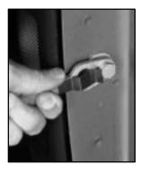
Raise the tailgate slightly and release both retaining cable clips.
