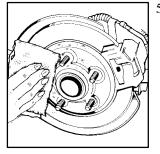
5. Remove any rust or dirt from the wheel bolts, mounting surfaces and spare wheel.
