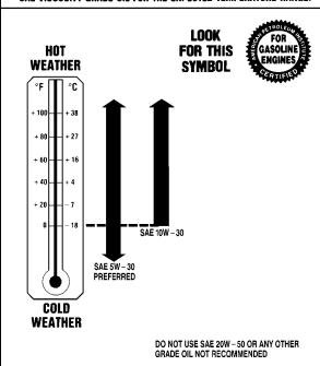
As in the chart shown previously, SAE 5W-30 is best for your vehicle. However, you can use SAE 10W-30 if it's going to be 0°F (-18°C) or above. These numbers on an oil container show its viscosity, or thickness. Do not use other viscosity oils, such as SAE 20W-50.
