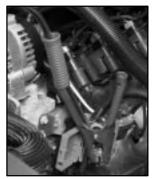
7. Connect the red positive (+) cable to the positive (+) terminal of the vehicle with the dead battery. Use a remote positive (+) terminal if the vehicle has one.
