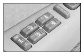
If your vehicle is equipped with power windows, the controls are located on each of the side doors in the front and rear.
