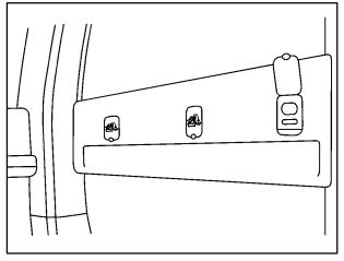
If your vehicle is a Crew Cab model, you'll find top strap anchors for the rear seating positions located on the back panel of your vehicle, behind the rear seat.
