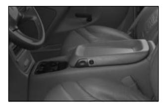
To open it, insert the console key into the lock and unlock the console. Press the button and swing the console lid open. The console has a place to store tissues, pens and a clip to hold business cards.
