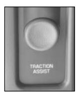
To turn the system on or off press the TAS on/off button located to the left of the steering wheel on the instrument panel.
