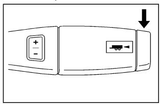
Vehicles with an Allison or Hydra-Matic<sup>®</sup> 6-speed automatic transmission<sup>®</sup> have a tow/haul mode. The tow/haul mode adjusts the transmission shift pattern to reduce shift cycling, providing increased performance, vehicle control, and transmission cooling when towing or hauling heavy loads. Turn the tow/haul mode on and off by pressing the button, located on the end of the shift lever. When the tow/haul is on, a light on the instrument panel cluster will come on.
