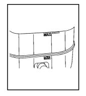
The fluid level should be above MIN. If it is not, have the brake hydraulic system checked to see if there is a leak.
