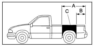
Use the rear edge of the load floor for measurement purposes. The recommended location for the cargo center of gravity is at point C for the CWR. It is the point where the mass of a body is concentrated and, if suspended at that point, would balance the front and rear. Here is an example of proper truck and camper match:
