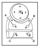
Vehicles with outside power foldaway mirrors have controls located on the driver door.
