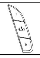
The controls for this feature are located on the driver's door panel, and are used to program and recall memory settings for the driver's seat, outside mirrors, and the adjustable throttle and brake pedal.
