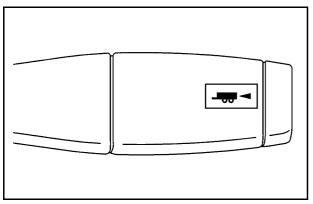
Vehicles with an automatic transmission have a tow/ haul mode. The tow/haul mode adjusts the transmission shift pattern to reduce shift cycling, providing increased performance, vehicle control, and transmission cooling when towing or hauling heavy loads.
