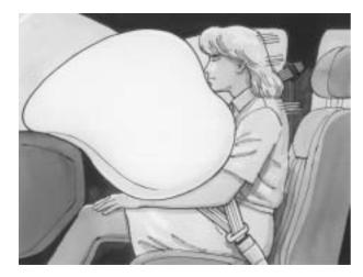
The right front passenger airbag is in the instrument panel on the passenger's side.
