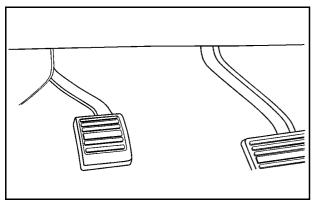
Set the parking brake by holding the regular brake pedal down, then pushing down the parking brake pedal. If the ignition is on, the brake system warning light will come on. See *Brake System Warning Light on page 4-39*.
