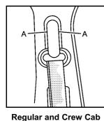
To move the adjuster down for the regular and crew cabs, squeeze the buttons (A) on the sides of the height adjuster and move the height adjuster to the desired position.
