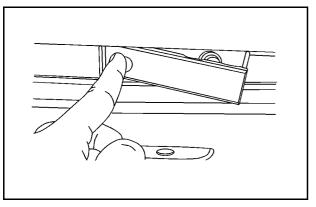
Access the storage area by pressing and holding in the driver side of the handle and pull out on the exposed portion of the handle.
