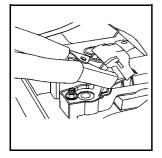
7. Connect the red positive (+) cable to the positive (+) terminal of the vehicle with the dead battery.
