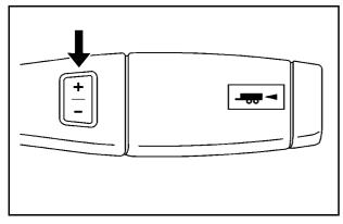
The Range Selection Mode switch is located on the shift lever. To enable the Range Selection feature, move the column shift lever to the M (Manual) position. The current range will appear next to the M. This is the highest attainable range with all lower gears accessible. As an example, when 4 (Fourth) gear is selected, 1 (First) through 4 (Fourth) gears are available.
