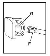
Insert the hoist end (open end) (F) of the extension through the hole (G) in the rear bumper.
