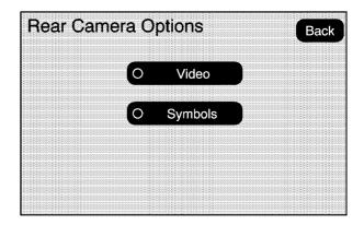
4. Select the Video screen button. When the Video screen button is highlighted the RVC system is on.
