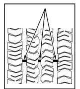
One way to tell when it is time for new tires is to check the treadwear indicators, which appear when your tires have only 1/16 inch (1.6 mm) or less of tread remaining. Some commercial truck tires may not have treadwear indicators. You need new tires if any of the following statements are true:
