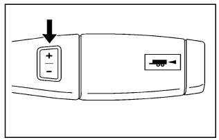
The vehicle may have a Range Selection Mode. The Range Selection Mode helps control the vehicle's transmission and vehicle speed while driving down hill or towing a trailer by letting you select a desired range of gears. To use this feature, do the following:
