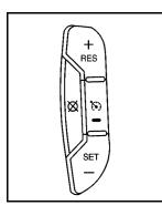
The cruise control buttons are located on left side of the steering wheel.
