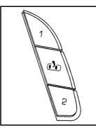
The controls for this feature are located on the driver door, and are used to program and recall memory settings for the driver seat, outside mirrors, and the adjustable throttle and brake pedal feature.
