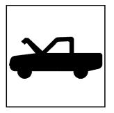
1. Pull the handle with this symbol on it. It is located inside the vehicle to the left of the brake pedal.
