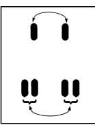
If your vehicle has dual rear wheels and the tread design for the front tires is different from the dual rear tires, always use the correct rotation pattern shown here when rotating the tires.
