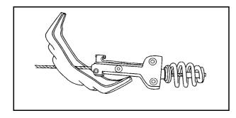
2. Separate the tire/wheel retainer (D) from the guide pin. Pull the pin through the center of the wheel. Tilt the retainer down and through the center wheel opening.
