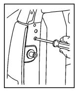
2. Remove the two rear lamp assembly screws near the tailgate latch strikerpost and pull out the lamp assembly.
