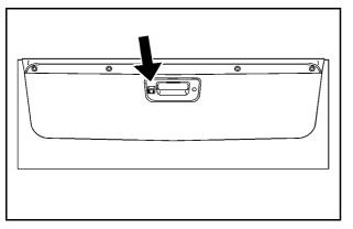
The image is provided by the camera located in the bezel for the tailgate handle.
