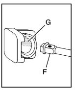
Insert the hoist end (F) through the hole (G) in the rear bumper and onto the hoist shaft.
