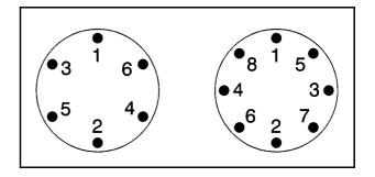
13. Tighten the nuts firmly in a crisscross sequence as shown by turning the wheel wrench clockwise.
