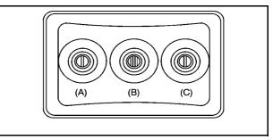
The A/V jacks, located on the rear of the floor console, allow audio or video signals to be connected from an auxiliary device such as a camcorder or a video game unit to the RSE system. Adapter connectors or cables (not included) may be required to connect the auxiliary device to the A/V jacks. Refer to the manufacturer's instructions for proper usage.
