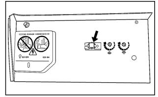
Locate in the garage, the garage door opener receiver (motor-head unit). Locate the "Learn" or "Smart" button. It can usually be found where the hanging antenna wire is attached to the motor-head unit and may be a colored button. Press this button. After pressing this button, complete the following steps in less than 30 seconds.
