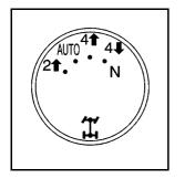
This transfer case knob is located next to the steering column.
