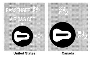
If the vehicle does not have an airbag off switch, it may have a passenger sensing system. See *Passenger Sensing System on page 2-85*. This switch should only be turned to the off position if the person in the right front passenger position is a member of a passenger risk group identified by the national government as follows:
