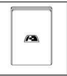
On vehicles with a power sliding rear window, the switch is located in the overhead console.
