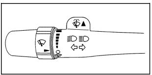
Turn the band with the wiper symbol to control the windshield wipers.
