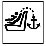
For regular cab models, there is an anchor symbol on the covers to assist you in locating the top tether anchors.
