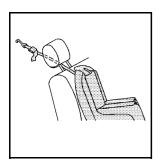
If the position you are using has an adjustable headrest or head restraint and you are using a single tether, raise the headrest or head restraint and route the tether under the headrest or head restraint and in between the headrest or head restraint posts.
