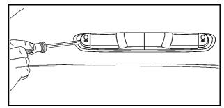
1. Remove the screws and lift off the lamp assembly.
