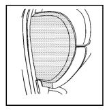
The instrument panel fuse block access door is located on the driver side edge of the instrument panel.
