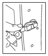
Raise the tailgate slightly and release both retaining cable clips. To release the retaining cable clips, lift the cable so it points straight out. Lift the clip over the bolt, and push the cable forward then rotate down. 2. With the tailgate about halfway open, lift the right edge of the tailgate from the lower pivot.
