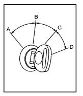
The ignition switch has four different positions.
