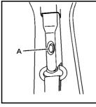
On the extended cab, push down on the release button (A) and move the height adjuster to the desired position.
