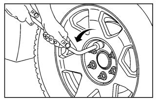
If the wheel has a smooth center cap, place the chisel end of the wheel wrench in the slot on the wheel, and gently pry it out. 3. Use the wheel wrench and turn it counterclockwise to loosen the wheel nuts. Do not remove the wheel nuts yet.
