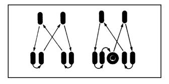
If your vehicle has dual rear wheels and the tread design for the front tires is the same as the rear tires, always use one of the correct rotation patterns shown here when rotating the tires.
