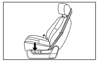
If equipped, the power seat controls are located on the outboard side of the front seats.
