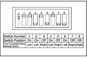
Example of Eight Dip Switches with Two Positions
