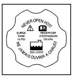
Remove the coolant surge tank pressure cap when the cooling system, including the coolant surge tank pressure cap and upper radiator hose, is no longer hot. Turn the pressure cap slowly counterclockwise about one full turn. If you hear a hiss, wait for that to stop. A hiss means there is still some pressure left.
