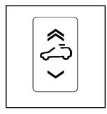
If your vehicle is an extended cab, the sunroof switch is located on the headliner above the rearview mirror. **Vent:** From the closed position, press and hold the rear of the switch to vent the sunroof. To close the sunroof, press and hold the front of the switch.
