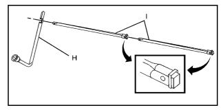
3. Attach the wheel wrench (H) and extensions (I) together, as shown.
